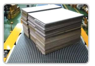
$\bullet$  TURN TABLE FOR  $0^{\circ} \sim 360^{\circ}$  STACK TURN WITHOUT STACK STOPPING
